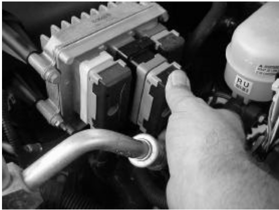
Fig # 5 reinstalling factory harness
